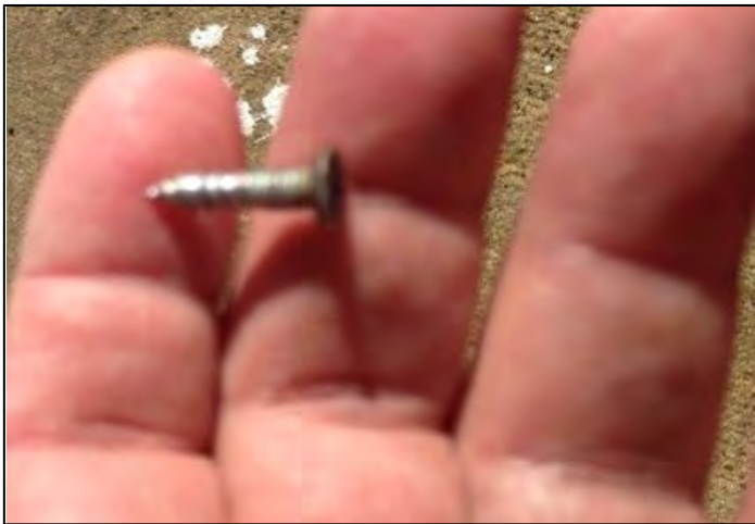
Typical 3/8" screw supplied with a doorknob kit
