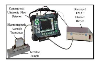
Ultrasonic flaw Detector are extremely used for the detection of flaw, and crack detection in the field of Nondestructive testing (NDT) of material.
