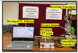
3. PC-based control automation and analysis software for ultrasonic pulse velocity tester with automatic threshold error correction
