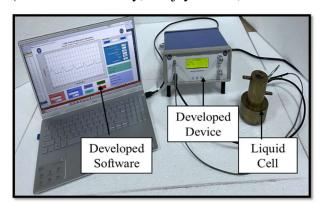
Ultrasonic interferometers are used for the ultrasonic velocity measurement in liquids.
