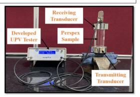
2. PC based ultrasonic pulse velocity tester with automatic threshold error correction (Team: P. K. Dubey, Sanjay Yadav, Ravinder Kumar, <u>Pivush</u>)
