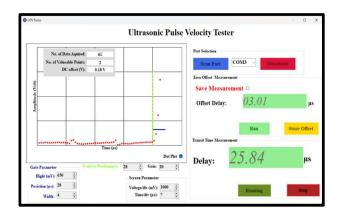
The developed software has the capability to analyze received ultrasonic analog signals and to measure ultrasonic transit time while also offering automatic threshold error correction.
