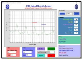
The sweep frequency ultrasonic interferometer software provides graphical images of the maxima and minima obtained in the liquid sample as well as the value of the ultrasonic propagation velocity. The response of the transducer disc can also be determined with this software.
