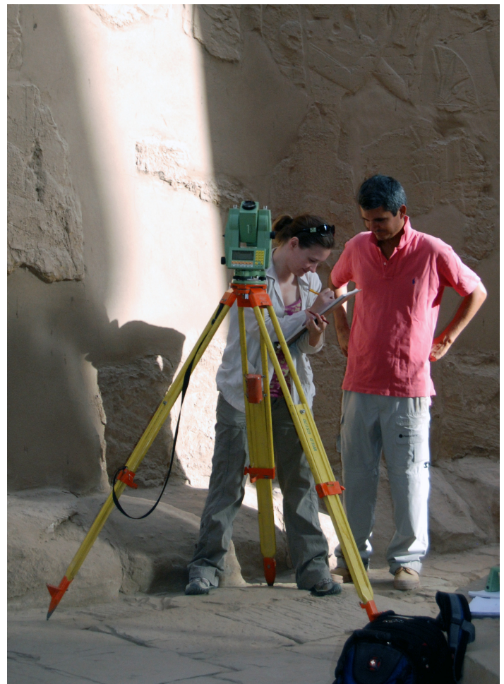
Molly Haight and Dr. Cédric Gobeil (Université de Québec à Montréal) using a laser theodolite surveying device to measure inscriptions high on the walls and columns of the Hypostyle Hall
