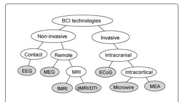
**Figure 1:** General classification of currently available brain activity monitoring BCI technologies. Technologies: EEG (Electroencephalography); MEG (Magnetoencephalography); MRI (Magnetic Resonance Imaging); fMRI (Functional MRI); dMRI (Diffusion MRI); DTI (Diffusion Tensor Imaging); ECoG (Electrocorticography); MEA (Multiple Electrode Array).
