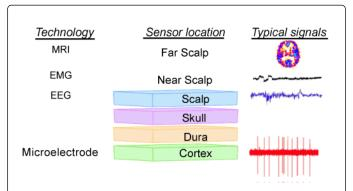
Figure 3: Typical signals for various BCI technologies and sensor location.
