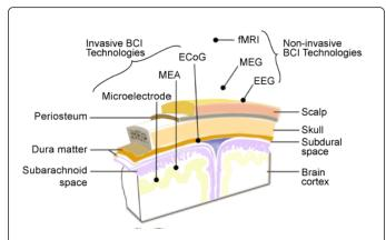
**Figure 2:** Typical electrode placement locations for various brain sensing technologies.
