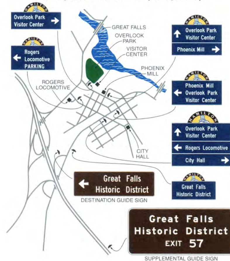
Figure 2D-19. Example of a Community Wayfinding Guide Sign System Showing Direction from a Freeway or Expressway
