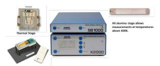
The system can provide information about the sign of the majority carrier, the mechanism of charge conduction, and in conjunction with appropriate theoretical models, information on the band structure of the material under investigation. Thermopower measurements are also an effective way of determining the intrinsic properties of samples having an electrical conductivity that is dominated by an extrinsic defect structure as
